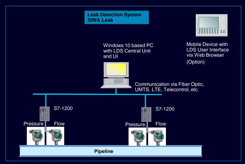
The leak monitoring system uses (the existing) flow and pressure instrumentation to detect and localize leaks.
