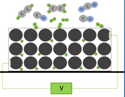
H<sub>2</sub> concentration as it permeates the proprietary solid-state substrate
